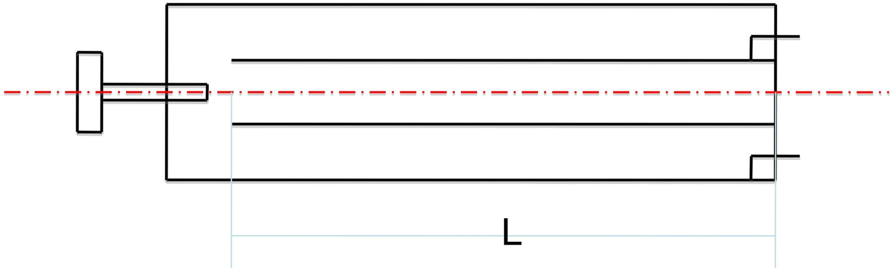
TEM mode,  $f \sim 350$  MHz. Low frequency structure usually for heavy ion (low beta) acceleration
